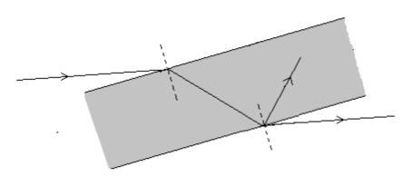
refracted emergent ray bent away from normal; angle of reflection equal to angle of incidence (by inspection); emergent ray parallel to original incident ray (by inspection);
