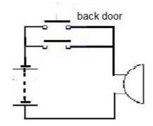
correctly placed second switch in parallel to first switch;
